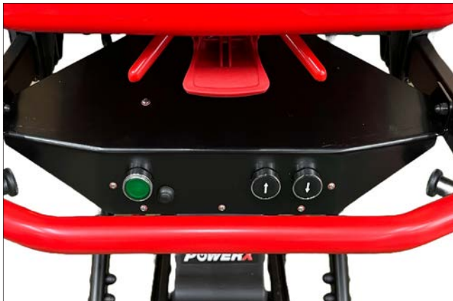
POWERX control box at foot-end
