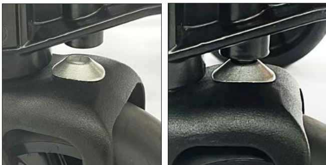
Directional wheel lock pin drops when engaged and locks into to of wheel fork once trolley is moved forward
