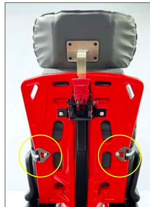
4-point harness attachment at back of backrest
