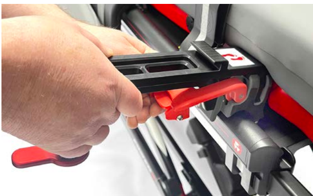
Attaching fixing bracket to siderail interface
