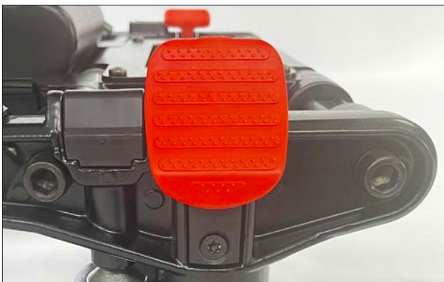
Wheel brake engaged, pedal points down
