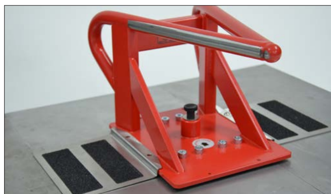
Plunger on SlideLock Spike
