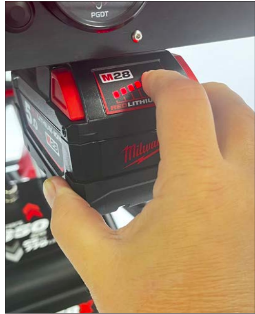
Battery LED charge status indicator
