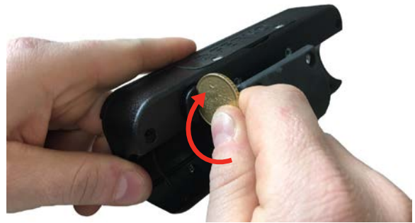
Opening the connector compartment
