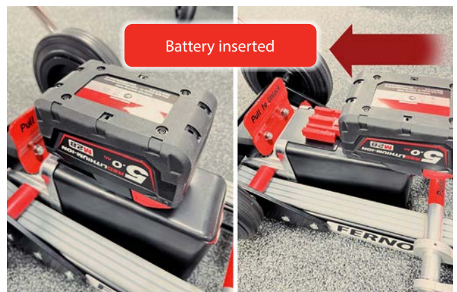
Battery attached to motor
