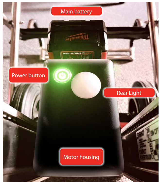
Main Battery & Motor Housing
