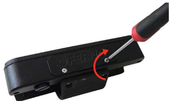
Opening the battery compartment
