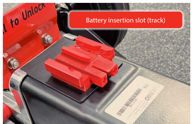
Battery holder on the track motor
