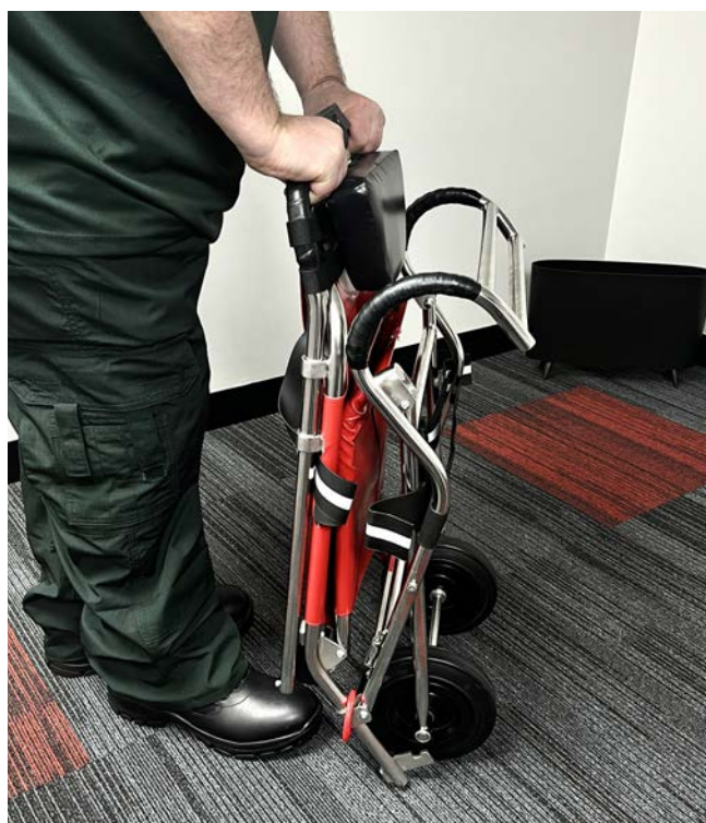
Chair folded and fastened secure for stowage
