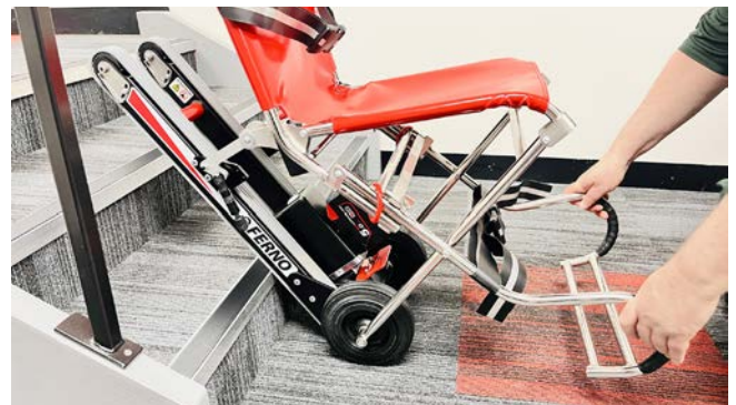
Tip the chair upwards whilst using the "+" button to bring the chair nearer to the bottom step, to then give more room to manoeuvre around the landing
