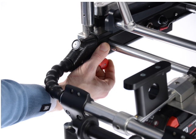
Figure 34 - Release by pulling plunger on rear of block
