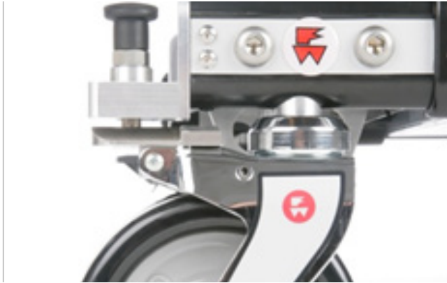
Figure 38 - Position location pin to apply wheel lock
