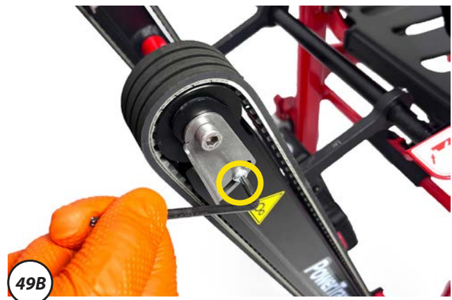
Figure 49 - Procedure for slackening the track tensioner
