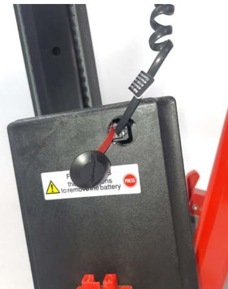
Figure 58 - Connecting the cable to the connector compartment
