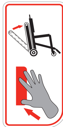
Instructions on how to close the track carriage
