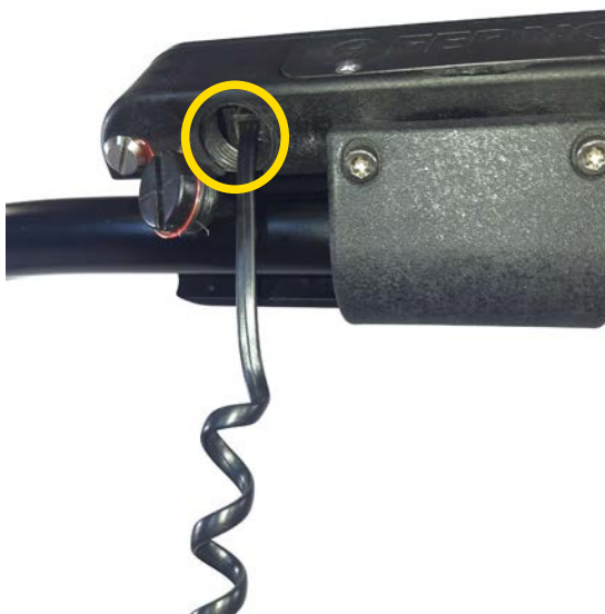
Figure 57 - Cable connected to the controller
