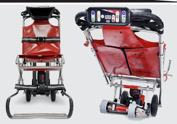
**Compact PowerTraxx** - a robust, lightweight and compact Powered Track Chair for transferring patients both up and down stairs, eliminating the need to lift, giving power-assistance to crews when moving up ramps and inclines, also contributing to an overall reduction in AMBULANCE vehicle weight.
