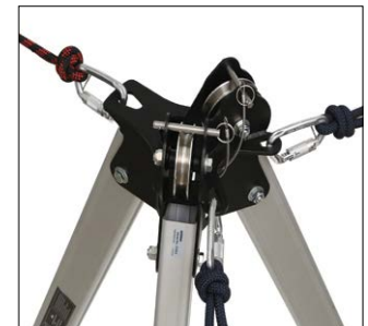
IndustriPOD+ with two 70mm sheave pulleys and pulley detent pins to prevent rope/cable jump
