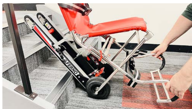
Tip the chair upwards whilst using the "+" button to bring the chair nearer to the bottom step, to then give more room to manoeuvre around the landing
