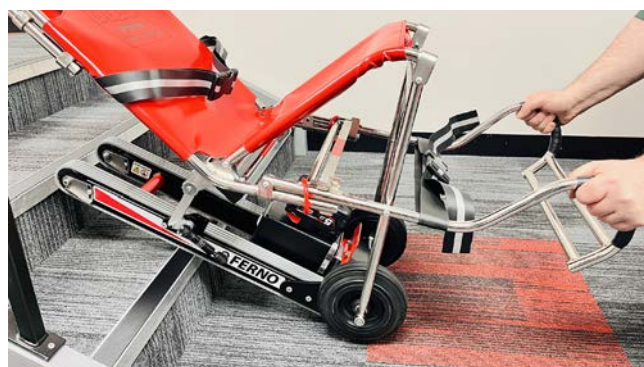
Stop as soon as wheels touch the landing floor
