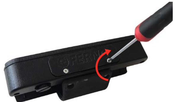
Opening the battery compartment
