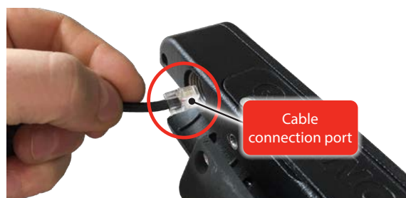
Connecting the cable to the connector port
