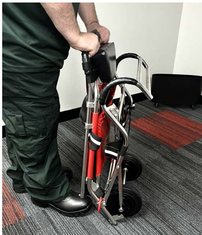
Chair folded and fastened secure for stowage
