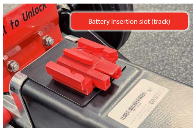
Battery holder on the track motor
