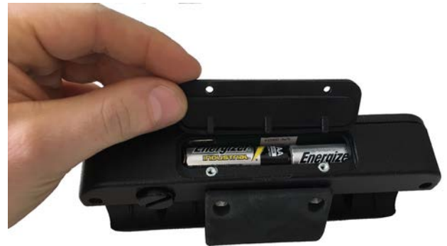
Opening the battery compartment
