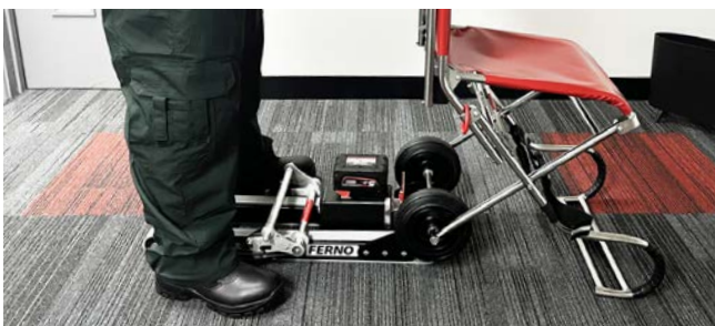
Push track towards chair to close the push-to-close latches and attach the track to the frame
