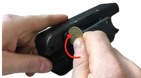
Opening the connector compartment
