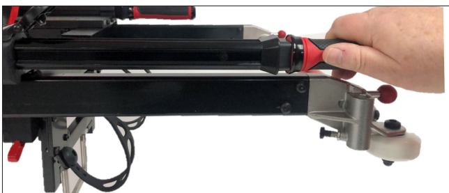
Push poles store discreetly inside the frame
