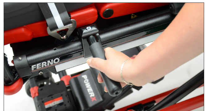
Unfold fully until clicks in place
