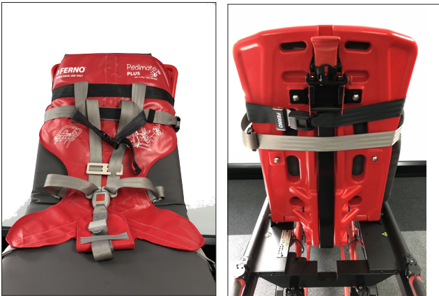
Attaching Pedimate top straps behind the backrest
