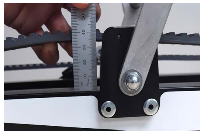
Fig 3 - place spacer between track module frame and track belt
