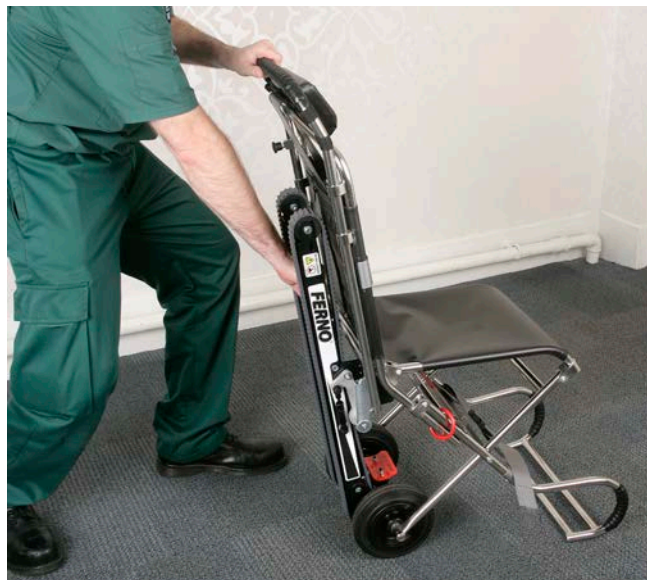
Figure 18 - Pulling Track out for use
