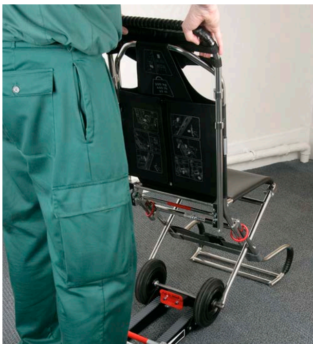
Figure 16 - Preparing to attach Track to unoccupied Chair
