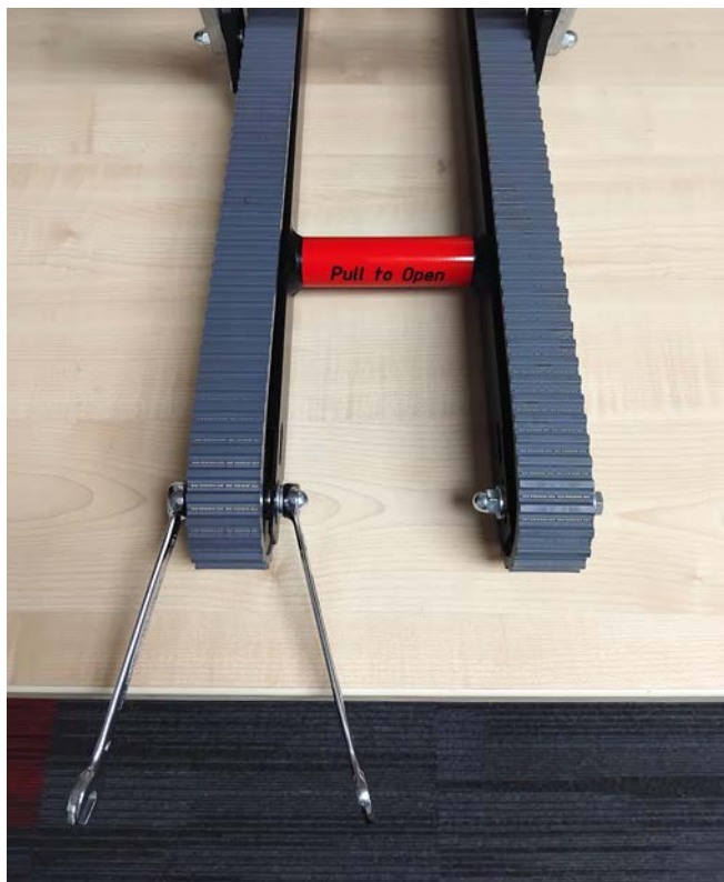
Fig 2 - loosening upper roller mounting bolt
