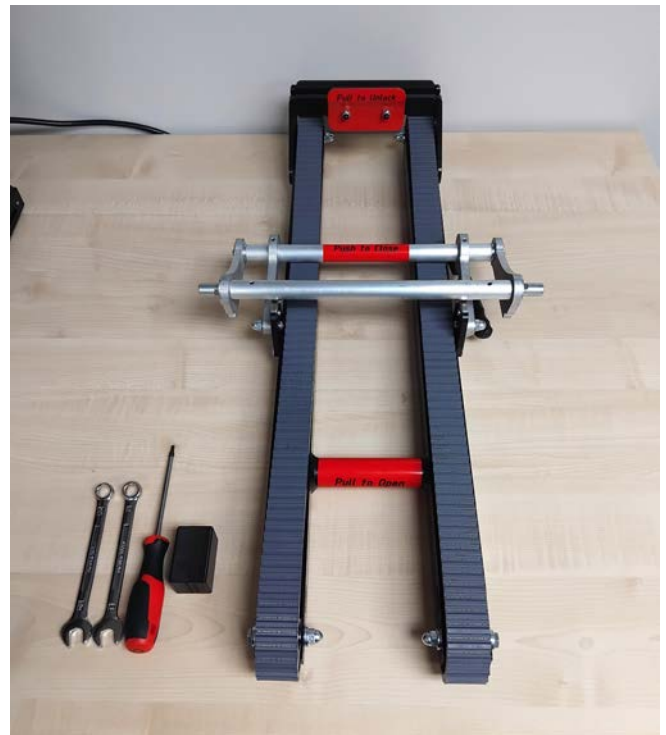
Fig 1 - place track on bench ready to check/adjust belt tension
