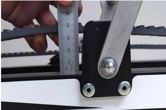
Fig 5 - Pull track belt upwards until no slack and measure distance
