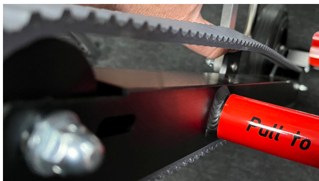
Detailed check, pulling the belt on top of track, the resulting gap between track and belt should be between 31 and 38 mm, 35 mm being the optimum
