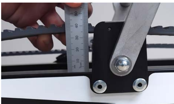
Detailed check, pulling the belt on top of track, the resulting gap between track and belt should be between 31 and 38 mm, 35 mm being the optimum
