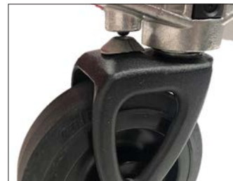
Directional wheel lock pin drops when engaged and locks into to of wheel fork once trolley is moved forward
