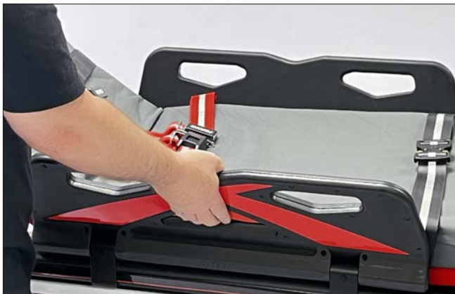
Squeeze the release lever
