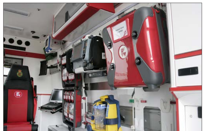
Ferno's IPTS iNTRAXX wall track bracket system
