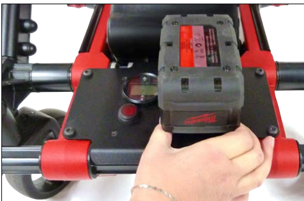
Removing battery pack
