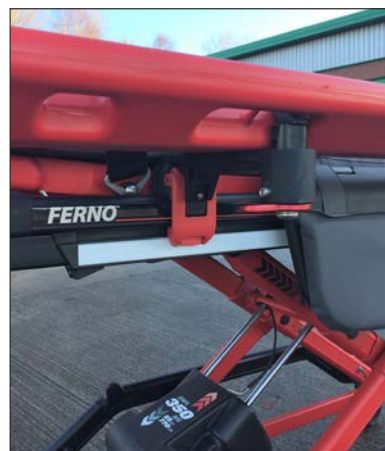
Locking device lever in full up position, locked
