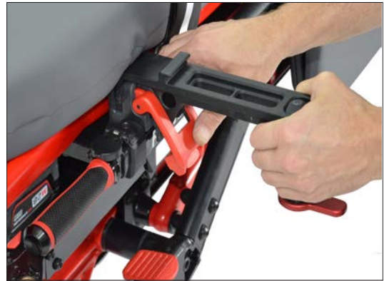
Lock the bracket in place by pressing down on the red locking handle until it clicks
