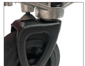
Directional wheel lock pin drops when engaged and locks into to of wheel fork once trolley is moved forward
