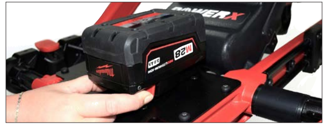
Removing battery pack
