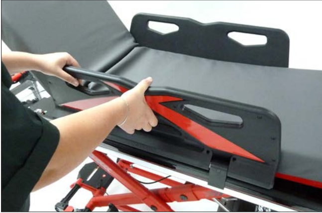
Squeeze the release lever
