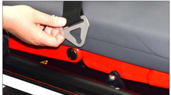
Strap tang with fixing hole
