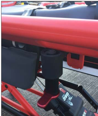
Locking arm unlocked
