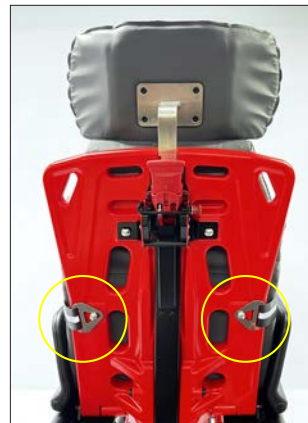
4-point harness attachment at back of backrest
