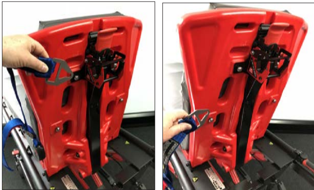
Attachment of upper ACR fixing straps to either set of fixing studs
