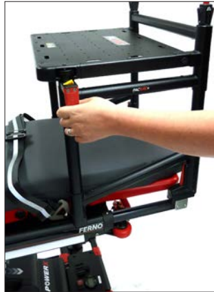
Twist the locking handle towards you
