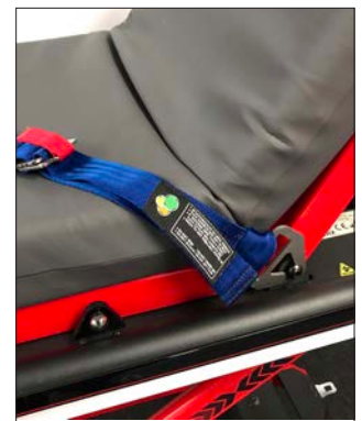
Attachment of lower ACR fixing straps to fixing stud at base of backrest either side of the trolley
