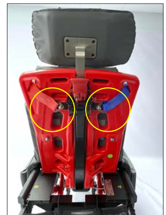
Cross-Strap harness attachment at back of backrest
