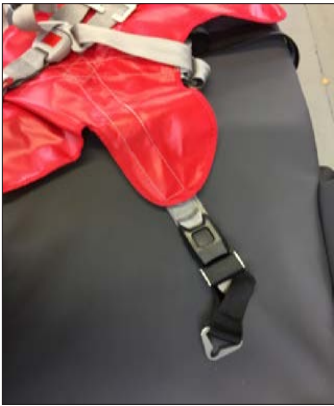
Loop strap and tang attached to PediMate fixing strap
