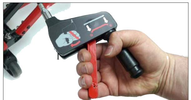
Gently squeezing the manual-over-ride handle to manually lower the trolley
