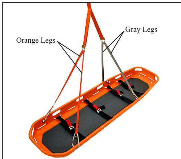
Figure 7 - Attaching the Orange and Gray Legs At Opposite Ends of the Stretcher
