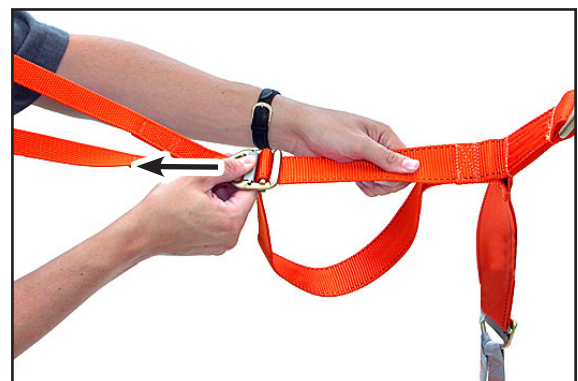
Figure 3 - Returning the Bridle To Full Length
