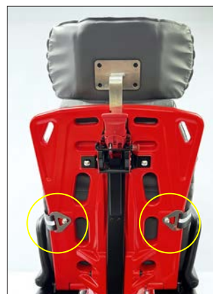
4-point harness attachment at back of backrest
