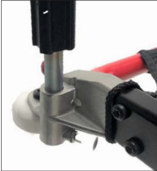
Insert push pole until it locks into place
