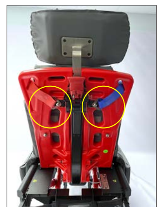
Cross-Strap harness attachment at back of backrest
