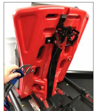
Attachment of upper ACR fixing straps to either set of fixing studs
