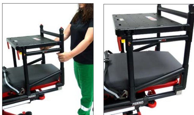
Sliding the PacRac+ onto the fixing points
