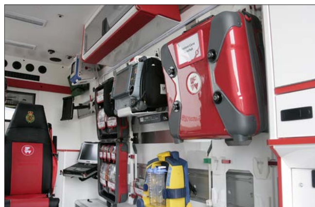
Ferno's IPTS INTRAXX wall track bracket system
