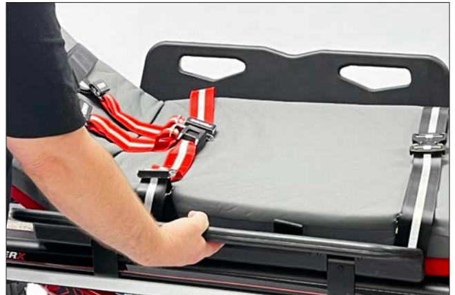
Moving SX cotside whilst depressing lever
