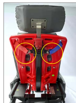
Cross-Strap harness attachment at back of backrest
