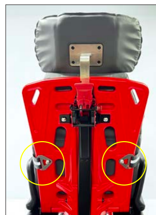
4-point harness attachment at back of backrest
