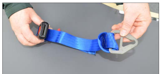
Attaching fixing tang to ACR blue fixing strap
