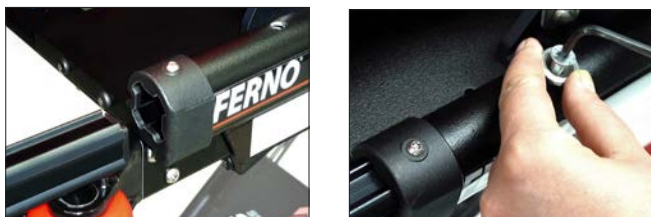
Attaching the fixing poles
