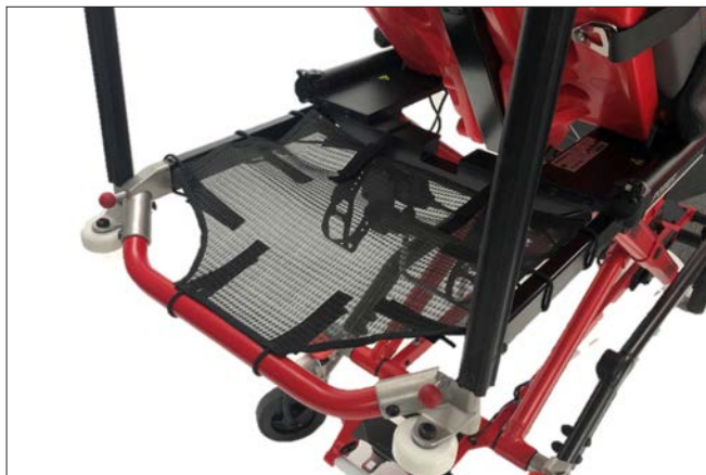
Storage net on head-end trolley frame
