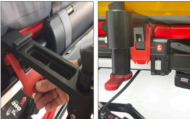
Attaching fixing bracket to siderail interface, LHS picture POWER Mkl at end, RHS picture MkII
