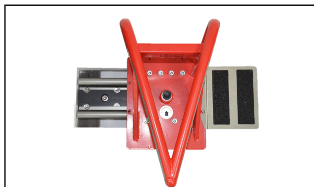
Removal of cover plates for cleaning linear slide rail and enclosure
