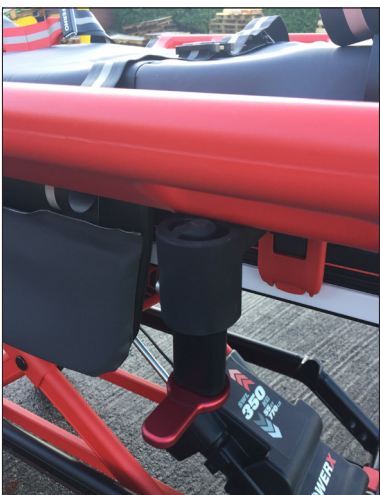
Locking arm unlocked
