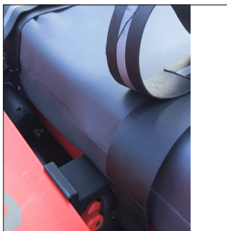
Ensure Scoop fins are positioned under the holding plates
