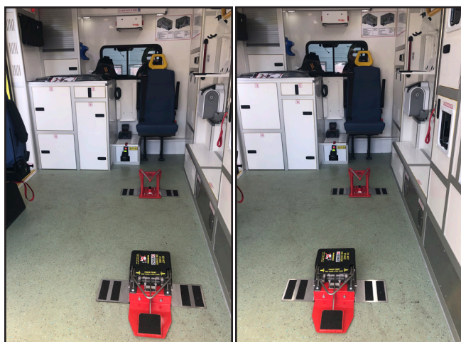
Foot-end SlideLock movement
