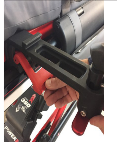
Lock the bracket in place by pressing down on the red locking handle until it clicks
