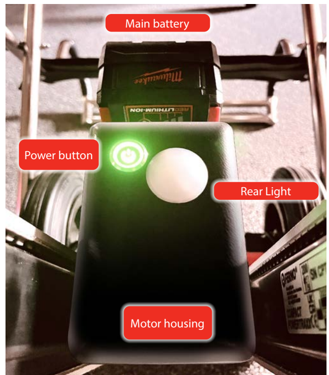
Main Battery & Motor Housing
