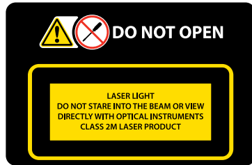
Do Not Open/Laser Notice Location: Controller Housing
